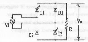
ii) In this single phase full converter T1 and T4 are given pulses at every ' $\alpha$ '. T2 and T3 are given pulses at every ' $\alpha + 180$ '. Unknowingly the gate pulses of T2 and T3 are removed and was given by the pulses of T1 and T2. Now explain, draw and derive the output voltage equation. (
